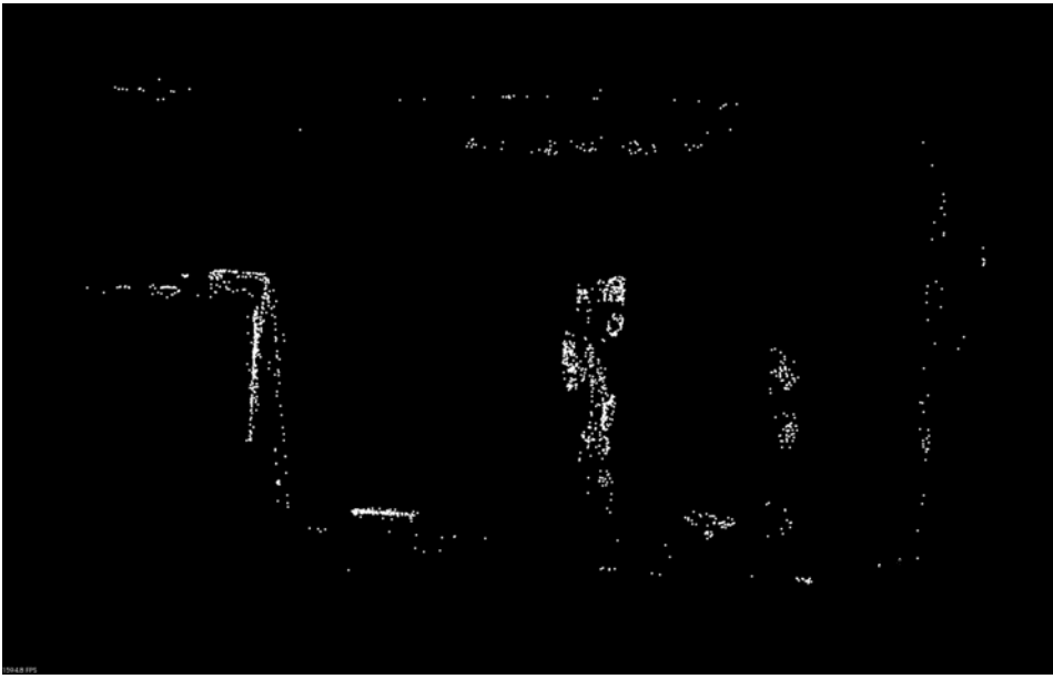
Figure 6.9 Keypoints from the keyframes using RANSAC and descriptor thresholding (1511 points).
