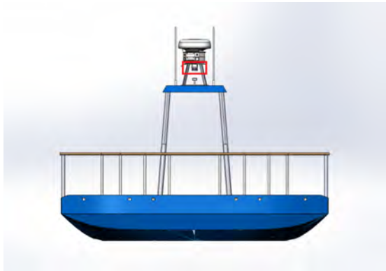
Fig. 5. Illustration of the ASV (MilliAmpere) used to record the data. The lidar is placed above the roof and is highlighted by the red square. Illustration created by Egil Eide.
